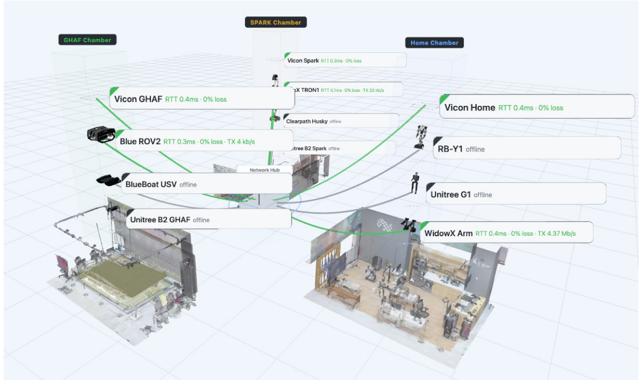
Figure 29: Fleet Networking dashboard—real-time network topology. Each robot is a node linked to its chamber; link color and animation encode latency, bandwidth, and connection state, and selecting a node reveals its live round-trip time, packet loss, and transmit rate.
